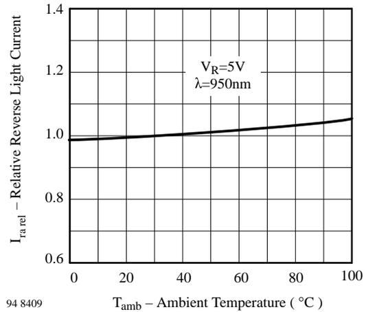
Figure 2. Relative Reverse Light Current vs. Ambient Temperature
