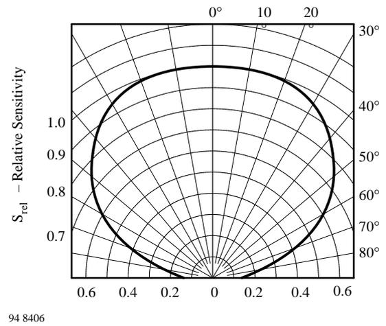
Figure 7. Relative Radiant Sensitivity vs. Angular Displacement
